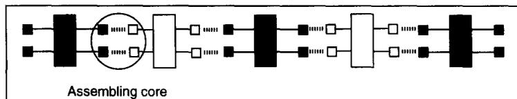
**Figure 1** : Schematic representation of an  $\alpha$ -network formed between complementary tectons. White and black squares represent H-bond donor and acceptor sites.
